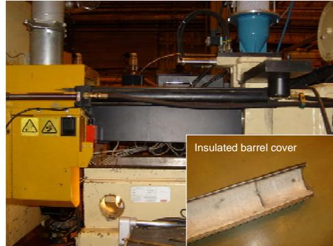
Figure 2. Induction Installation (nXheat™)
